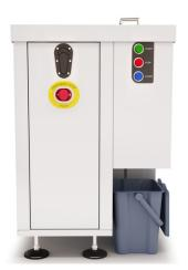
With the state-of-the-art B&M Food Waste Station Compact, food waste is macerated into a liquid form and pumped directly into a built-in de-watering system, forcing out excess liquid. This liquid is fed directly into the drain resulting in a greatly reduced volume of food waste, which is then collected in small, easily managed, lidded bins, ready for onward processing.
