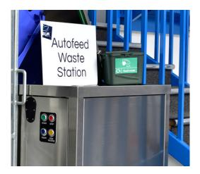
The B&M Waste Station Autofeed builds on the compact waste station and allows more than the single bucket feed of the Waste Station and Waste Station CR. Food waste is emptied into the collection chamber and auger fed into the maceration chamber before being pumped to the remote drying unit, which can be up to 55m away. This ensures maximum efficiency in busy kitchens / prep areas.
