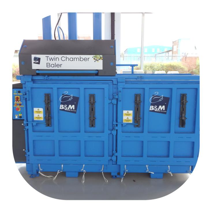
The B&M Twin Chamber Baler produces up to 200kg bales of cardboard or plastic film. Each material can be baled independently, negating the need to store quantities of material prior to baling.
