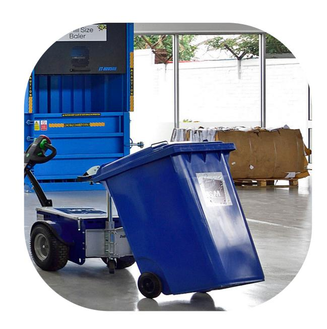
The B&M electric pedestrian tug is perfect for indoor and outdoor use. It is small, manoeuvrable and powerful enough to tow up to 3000KG. It has a range of up to 12 miles with a full loads on a single charge, with a recharge time of approximately 4 hours.
